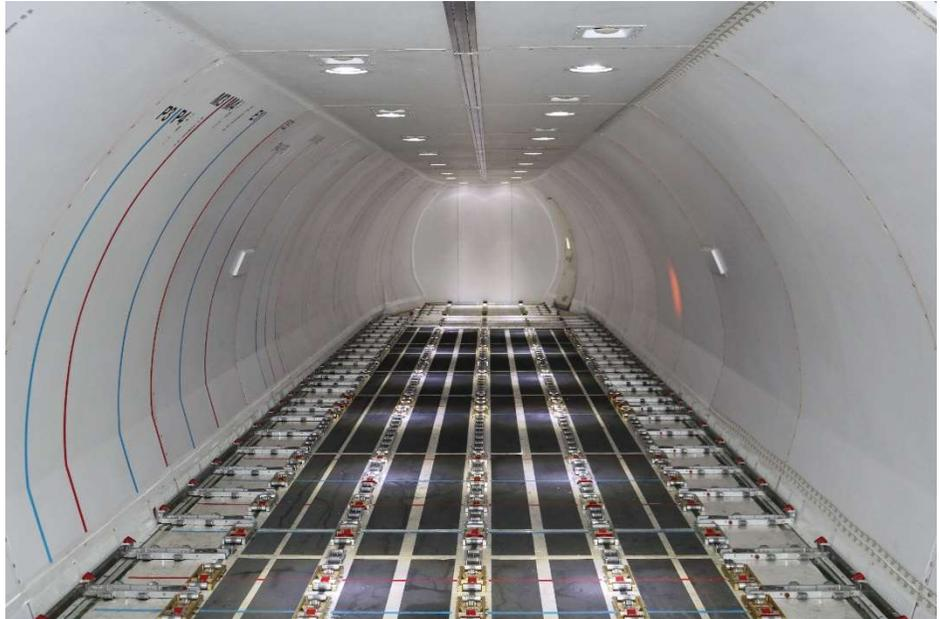
*The inside of an Alaska Airlines 737-700BDSF, equipped with an Ancra cargo loading system.*
